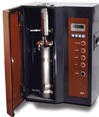
Abbildung 7: Electronic Low Pressure Impactor (Dekati Oy, Tampere)
