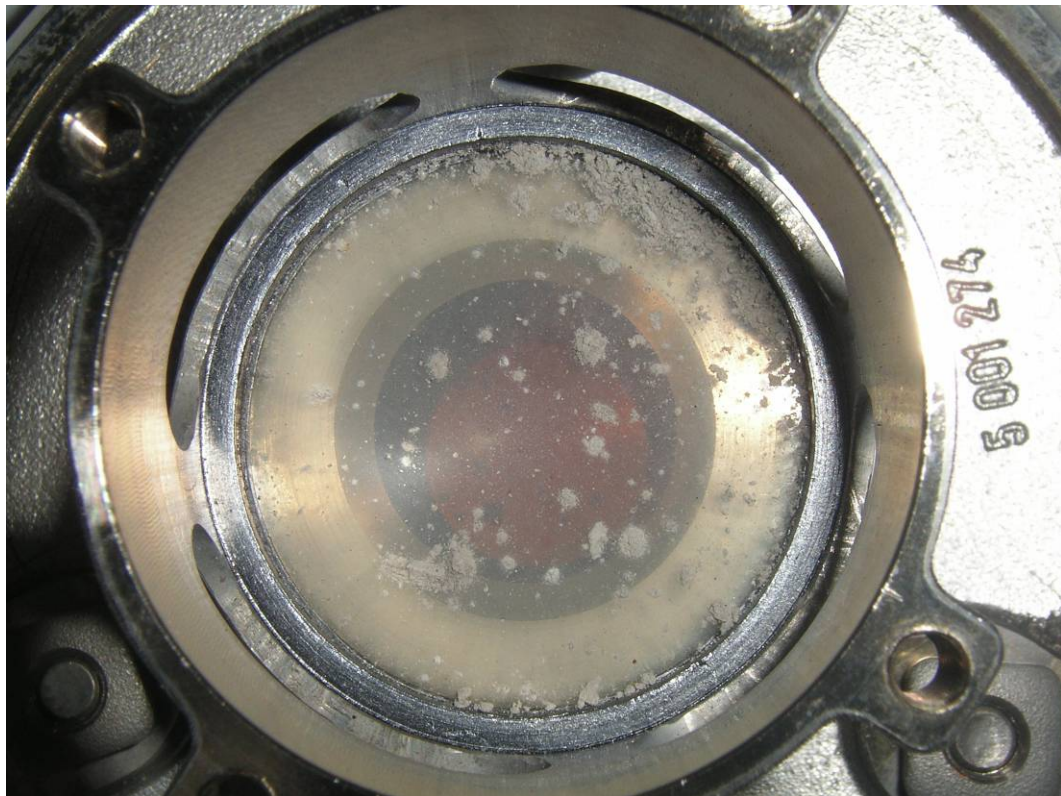
Figure 4.5: Sticking dust on the optic of the sonde
